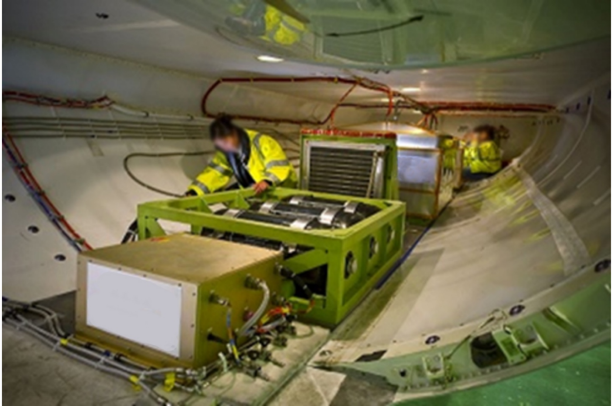
Figure 46. Regenerative FC Energy Storage System Demonstrator
