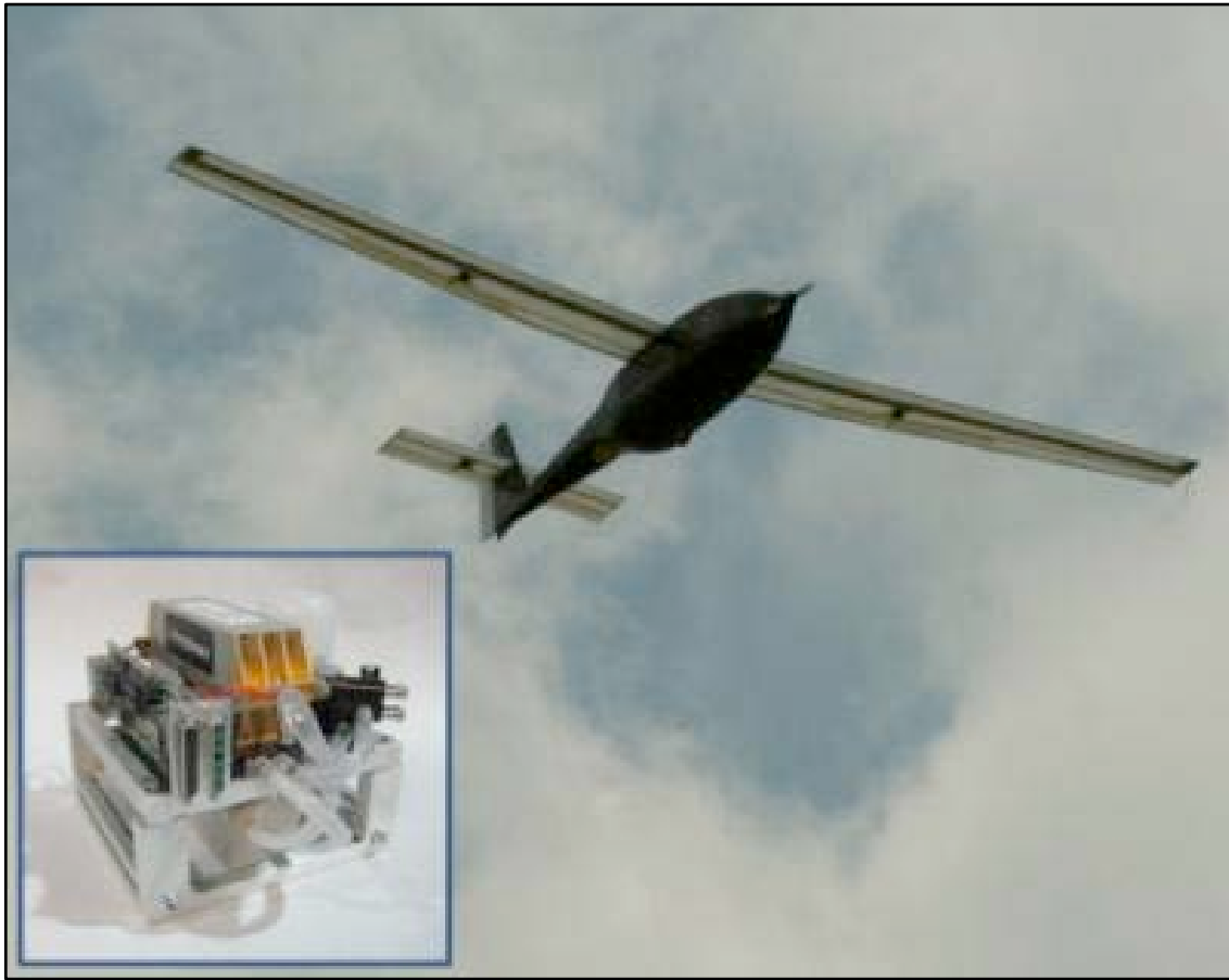
Figure 66. Ion Tiger Fuel Cell-Powered UAV
