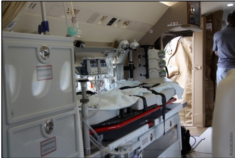
Figure 56. Dedicated Medevac Aircraft—On-Board Installation
