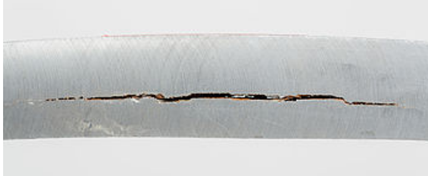
Figure 77. Hydrogen-Induced Cracks (HIC)
