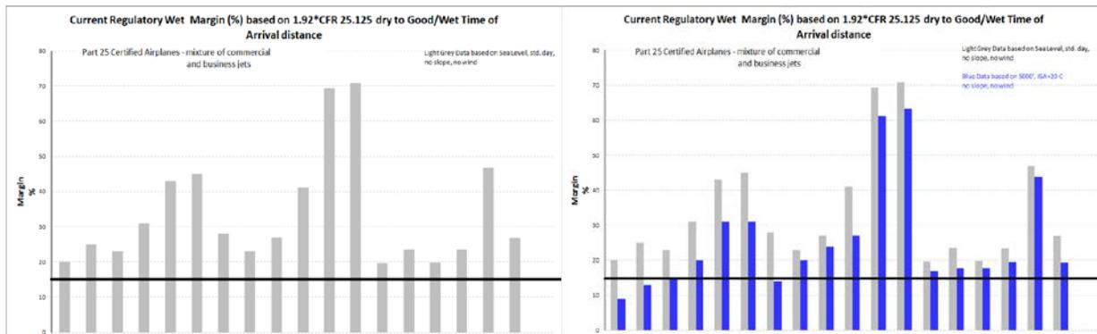
The grey is at Sea Level, Standard Day; the blue is at 5000' elevation ISA+20C (25C OAT), say a fall day in Denver. As can be seen the margin goes down significantly and if you go to 10000 feet it gets less yet. You can also see the variation in margin based on certification methods be it by company choice or certification agency
