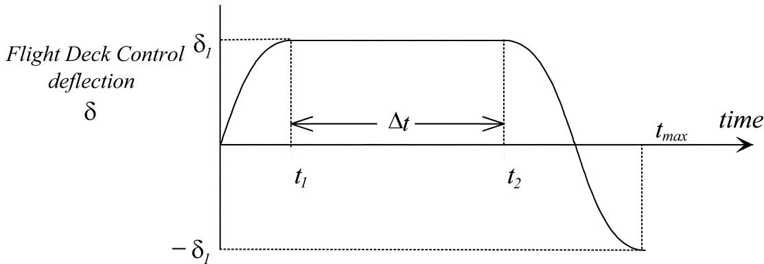
(iv) In cases where the flight deck pitch control motion may be affected by inputs from systems (for example, by a stick pusher that can operate at high load factor as well as at 1g), then the effects of those systems shall be taken into account.
