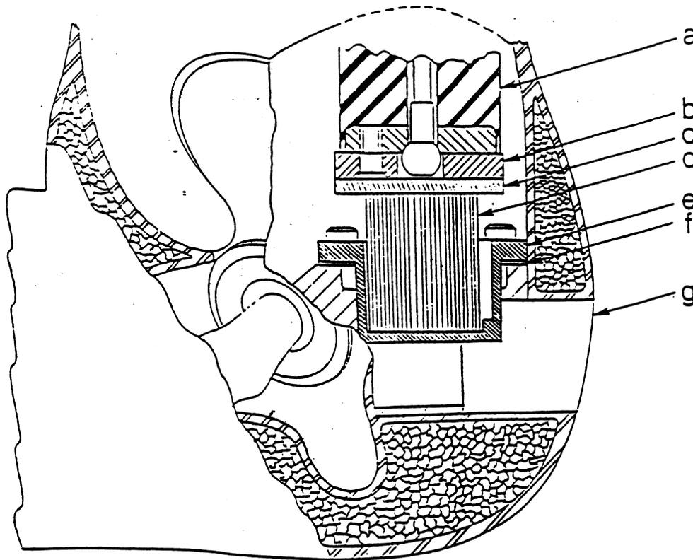
Figure 2. Installation of Pelvic-Lumbar Spine Load Cell
