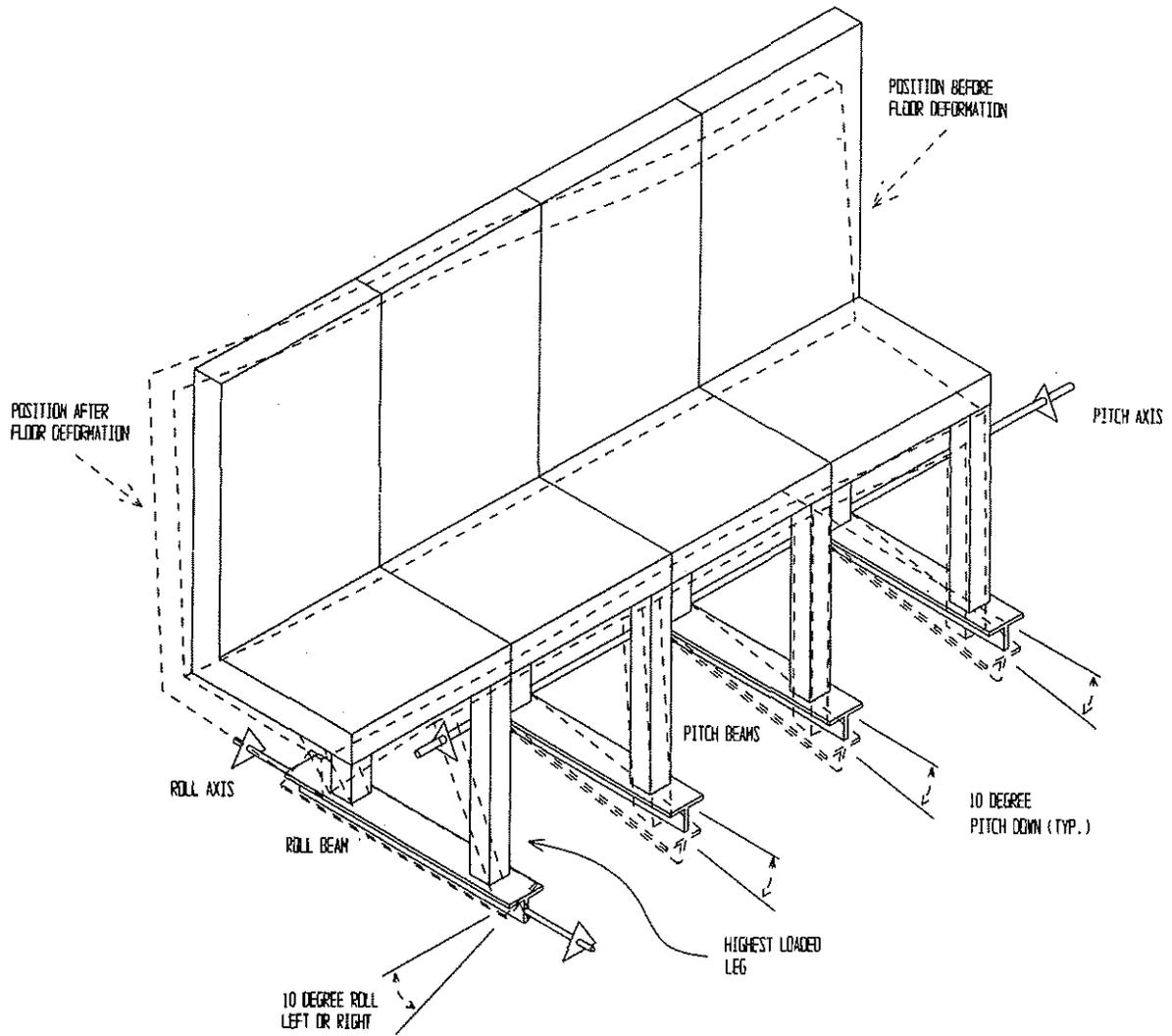
Figure 5. Floor Warpage Multiple Leg Seat
