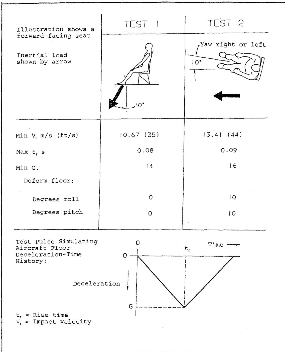
Figure 1. Type A Seat/Restraint System Dynamic Tests
