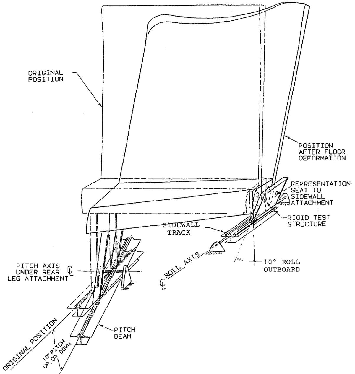
Figure 6. Schematic Test Fixture; Sidewall Mounted Seat
