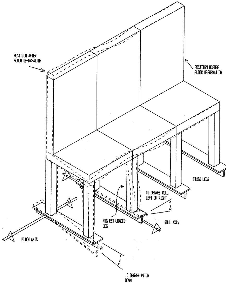
Figure 4. Floor Warpage Multiple Leg Seat
