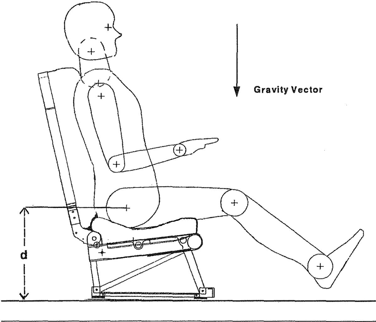
Figure 7. Measurement of 1g Preload
