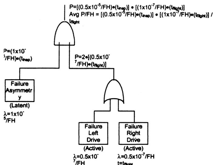
$$\{ [(1 \times 10^{-5} / FH \text{ Monitor Failure}) \cdot (t_{insp} \text{ hr dormancy period})] \cdot [(0.5 \times 10^{-7} / FH \text{ Either Drive Shaft Severance}) \cdot (t_{flight} \text{ hr avg flight})] \} / (t_{flight} \text{ hr avg flight}) < 1 \times 10^{-9} / FH$$
