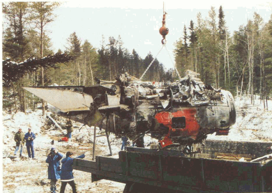
The aircraft was dismantled and transported to Ottawa for examination. These photographs show the left engine being removed and loaded onto a truck.
