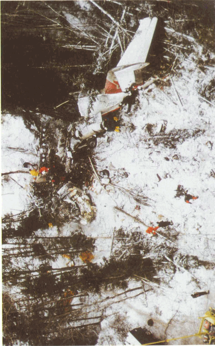
An aerial view of the wreckage of C-FONF, showing the aircraft in three pieces. The Air Ontario designator is clearly visible on the tail section.
