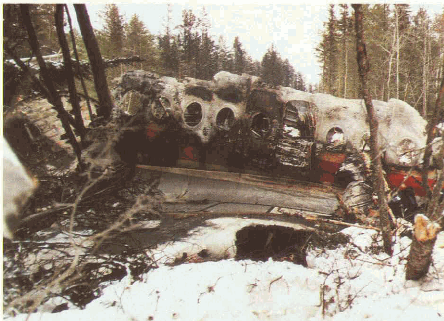
The wreckage was carefully photographed in situ at the crash site by the investigators: top, right engine; bottom, rear section of the right side of the fuselage.
