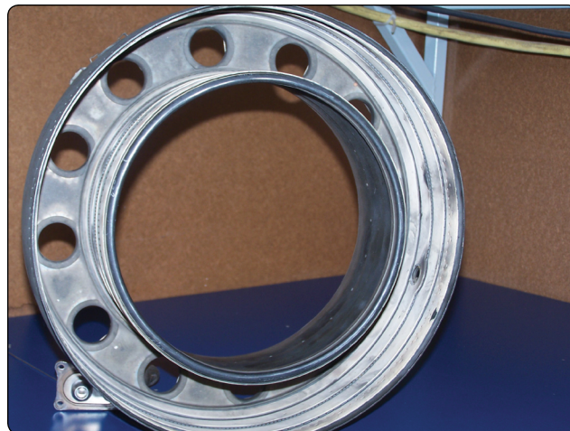
Figure 1-58. Annular combustion chamber with ceramic coating.
