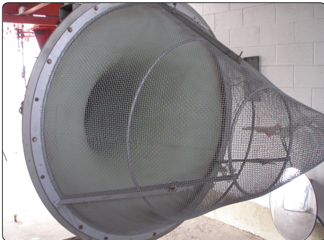
Figure 3-30. A bellmouth inlet used during system tests.
