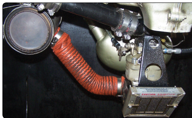
Figure 3-5. Location of a carburetor heat air valve.
