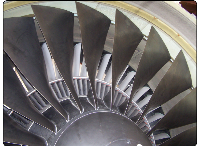
Figure 3-45. Fan air is directed through the fan blades and exit vanes.
