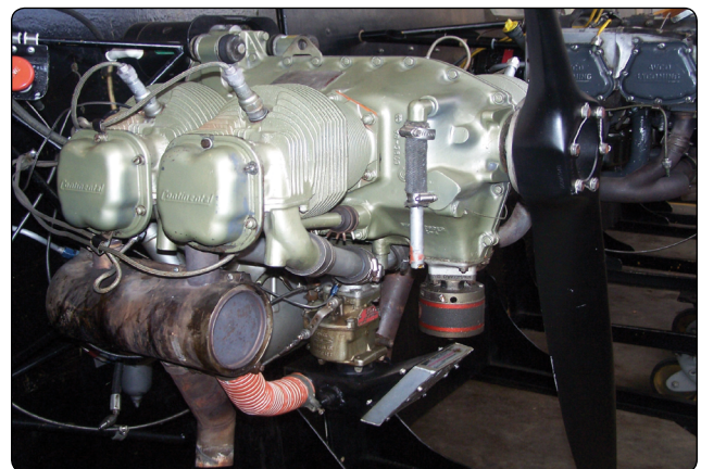
Figure 3-9. An example of a naturally aspirated reciprocating engine.
