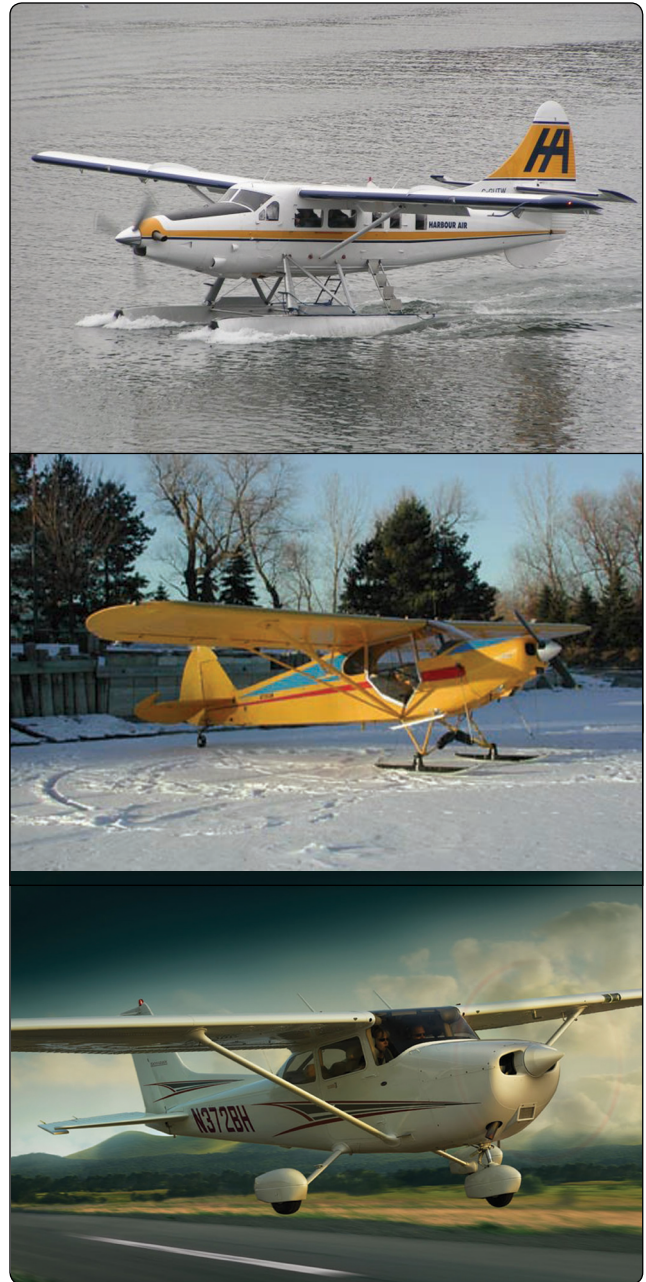
Figure 3-12. Types of landing gear: floats (top), skis (middle), and wheels (bottom).
