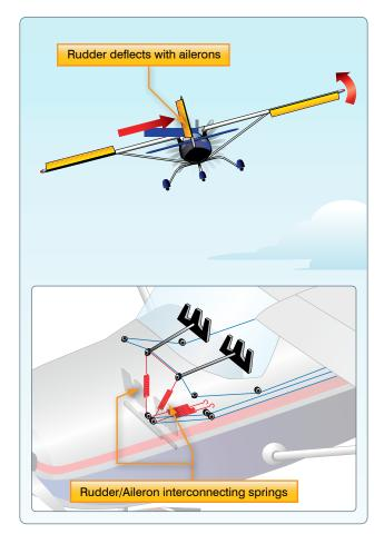
Figure 6-8. Coupled ailerons and rudder.
