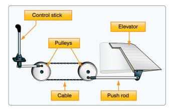
Figure 6-1. Mechanical flight control system.
