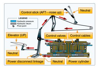
Figure 6-2. Hydromechanical flight control system.
