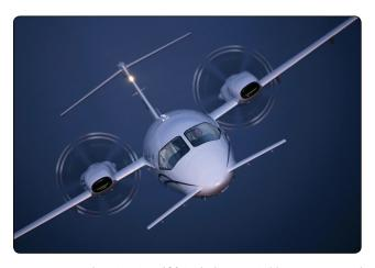
**Figure 6-14.** *The Piaggio P180 includes a variable-sweep canard design that provides longitudinal stability about the lateral axis.*
