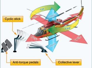
Figure 6-3. Helicopter flight control system.
