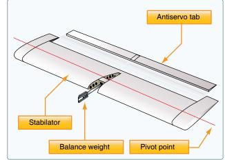
**Figure 6-13.** *The stabilator is a one-piece horizontal tail surface that pivots up and down about a central hinge point.*
