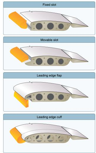
Figure 6-18. Leading edge high lift devices.
