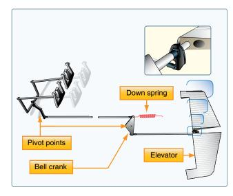
**Figure 6-12.** When the aerodynamic efficiency of the horizontal tail surface is inadequate due to an aft CG condition, an elevator down spring may be used to supply a mechanical load to lower the nose.
