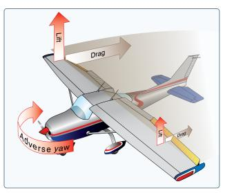
**Figure 6-5.** Adverse yaw is caused by higher drag on the outside wing that is producing more lift.
