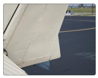
**Figure 6-22.** A ground adjustable tab is used on the rudder of many small airplanes to correct for a tendency to fly with the fuselage slightly misaligned with the relative wind.
