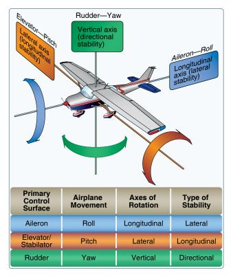
**Figure 6-4.** *Airplane controls, movement, axes of rotation, and type of stability.*
