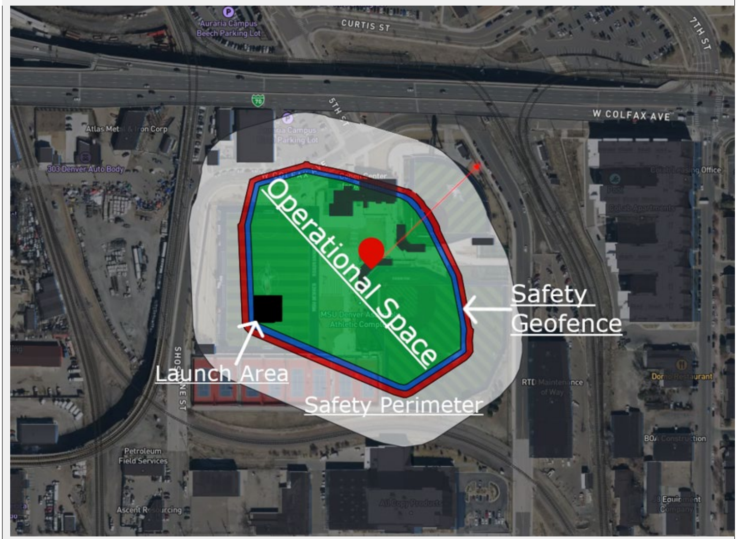
Figure 4: Additional Airspace / Site Assessment Screenshot
