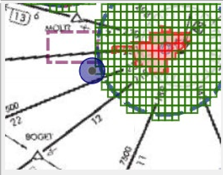
Figure 3: IFR Low Altitude Enroute Chart / UASFM Overlay
