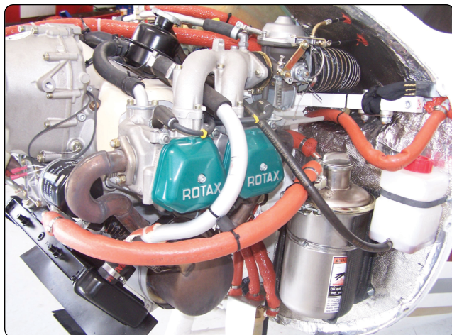
Figure 11-6. Typical four-cylinder, four-stroke horizontally opposed engine.
