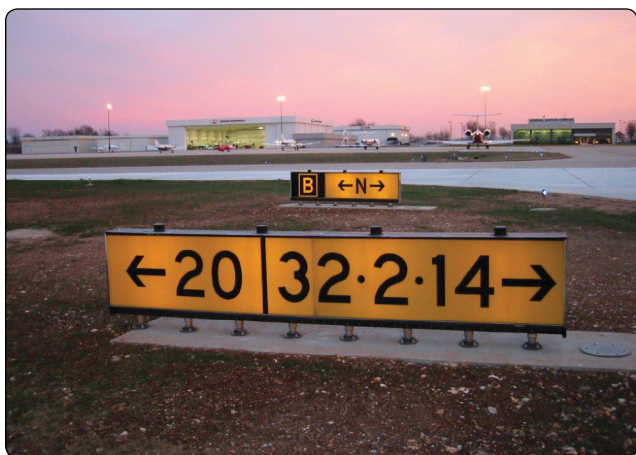
Figure 14-23. Runway destination sign with different taxi routes.
