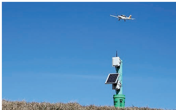
Stand-alone Version II device installed at Indianapolis Executive Airport (KTYQ) for data collection at a non-towered airport.
