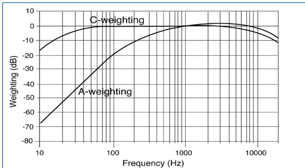
**Figure 2. Frequency Response Characteristics of A- and C-Weighting.**
