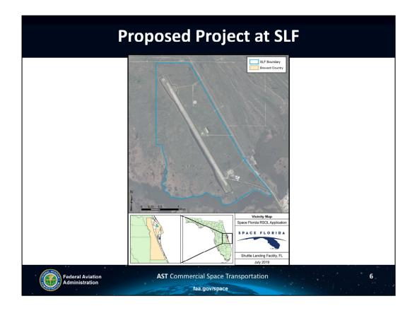
The image on this slide shows the reentry site boundary, circled in blue, around the SLF. The Dream Chaser would land on Runway 15/33 in an unpowered landing. Upon touch down, the vehicle would brake and come to a complete stop along the runway.
