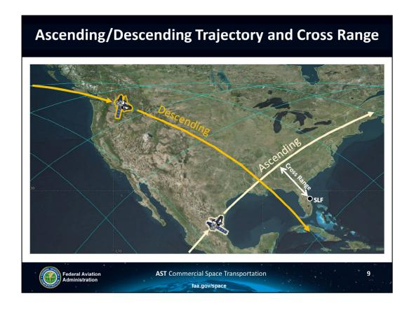
Some key terms used when describing the reentry of Dream Chaser are defined on this chart. Reentries can either be on ascending or descending trajectories, as shown in the image. Ascending is when the relative motion of the ground track projected by the orbiting vehicle is moving in an upward direction relative to the landing site. Descending is a downward motion relative to the landing site. For the proposed reentry to SLF, Sierra Space is proposing ascending trajectories.
