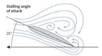
It is important for the pilot to understand that a stall is the result of exceeding the critical AOA, not of insufficient airspeed. The critical AOA is an aerodynamic constant for a given airfoil in a given configuration. The velocity of the relative wind does not matter; the airfoil will ALWAYS stall when the critical AOA is reached.
