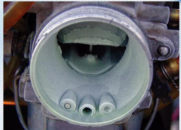
***An example of carburetor icing from a real incident that affected power significantly.***
