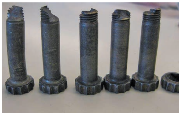
Broken Omega landing gear bolts.
