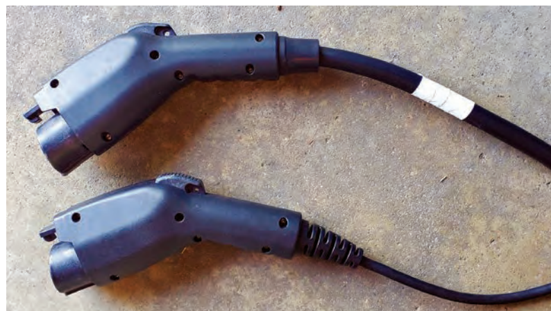
While both Level 1 and 2 use the same J-1772 connector, note the difference in cord gauge of the Level 2 connection on top. The 240V 32A EVSE requires a much heavier cord.
