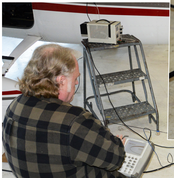
ADS-B ground testing equipment, as shown here, can verify all parameters are correct after an ADS-B installation.
