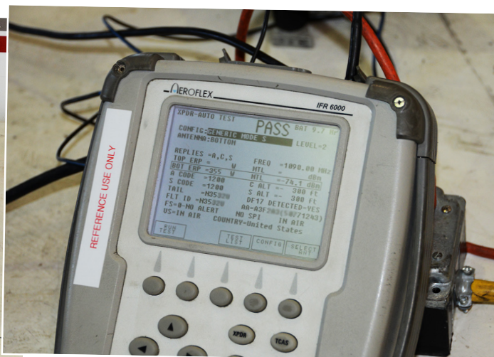
ADS-B ground testing equipment, as shown here, can verify all parameters are correct after an ADS-B installation.
