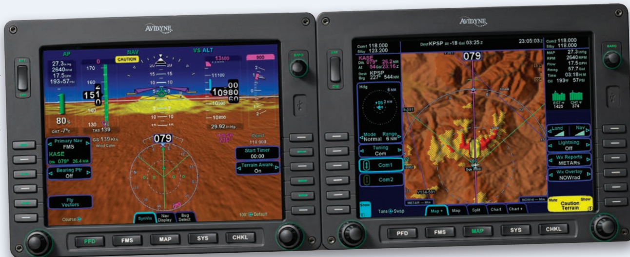
Synthetic vision displayed on a cockpit display.
