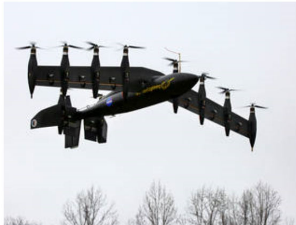
The GL-10 prototype takes off in hover mode like a helicopter. Credits: NASA Langley/David C. Bowman
