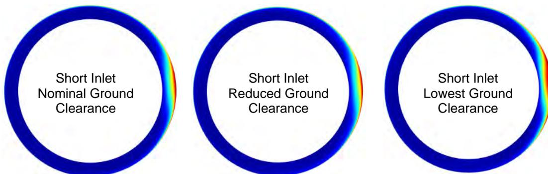
Figure 5-5. Rake total pressure contour, short inlet @ fan design speed, max blower speed, nominal (left), reduced (center) and lowest (right) ground clearance
