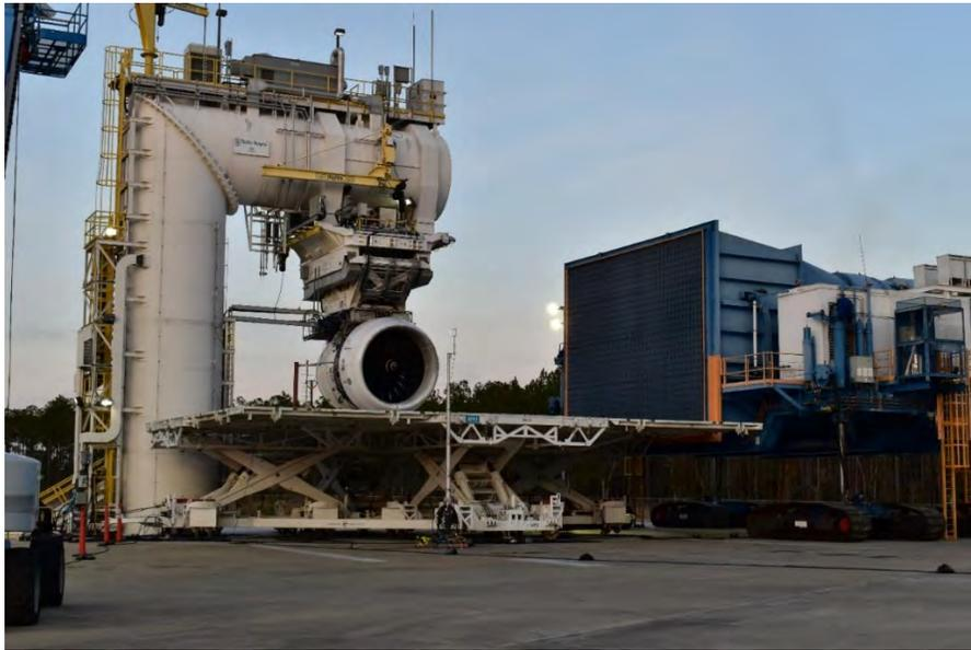
Figure 3-1. 90° crosswind setup on Bed 60 for Trent 1000 engine with the short inlet
