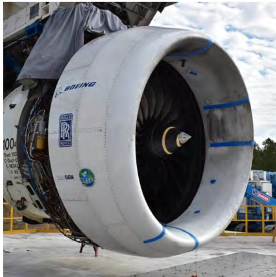
Figure 3-2. Short inlet installed on Trent 1000 engine
