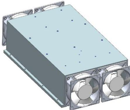
**Figure 6-5 – Heat Sink with fans**
