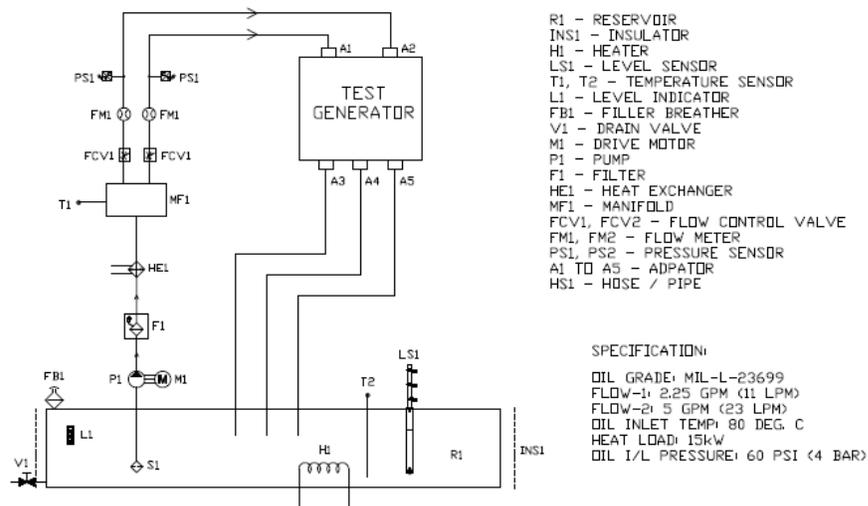
**Figure 6-2 - PID diagram of HPSG generator cooling**
