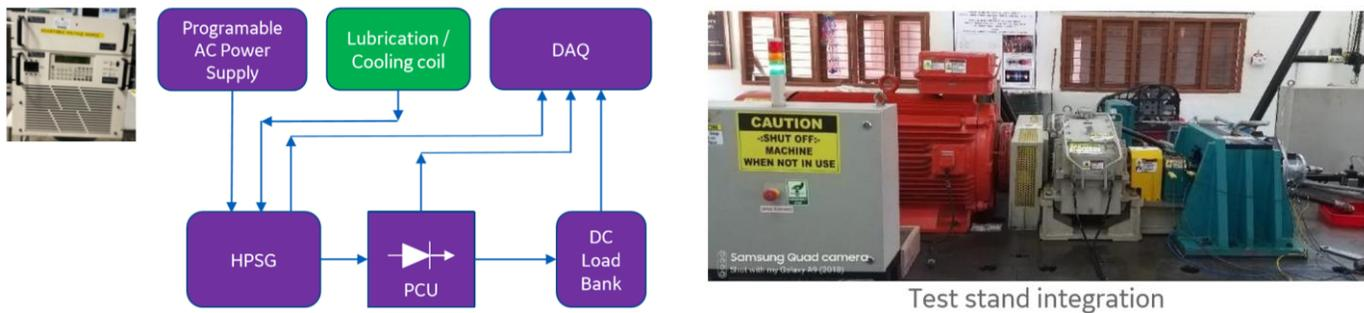
**Figure 6-3 - HPSG Component Testing**
