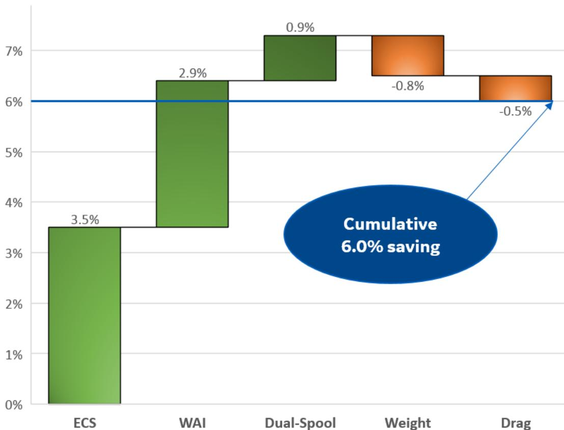
**Figure 4-1 - Breakdown of System Impact on Fuel Savings (500 NM, Icing Conditions)**
