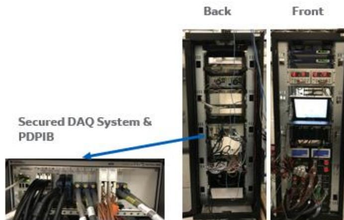
**Figure 7-3 - PDIPIB & DAQ Rack**
