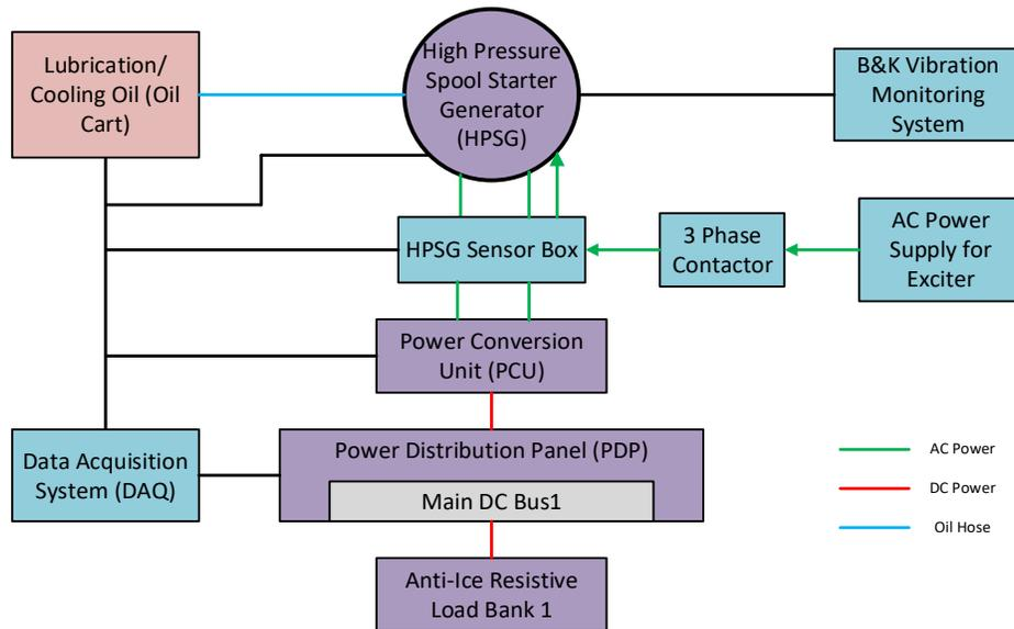
**Figure 7-9 – HPSG and PCU Open Loop Test block diagram**
