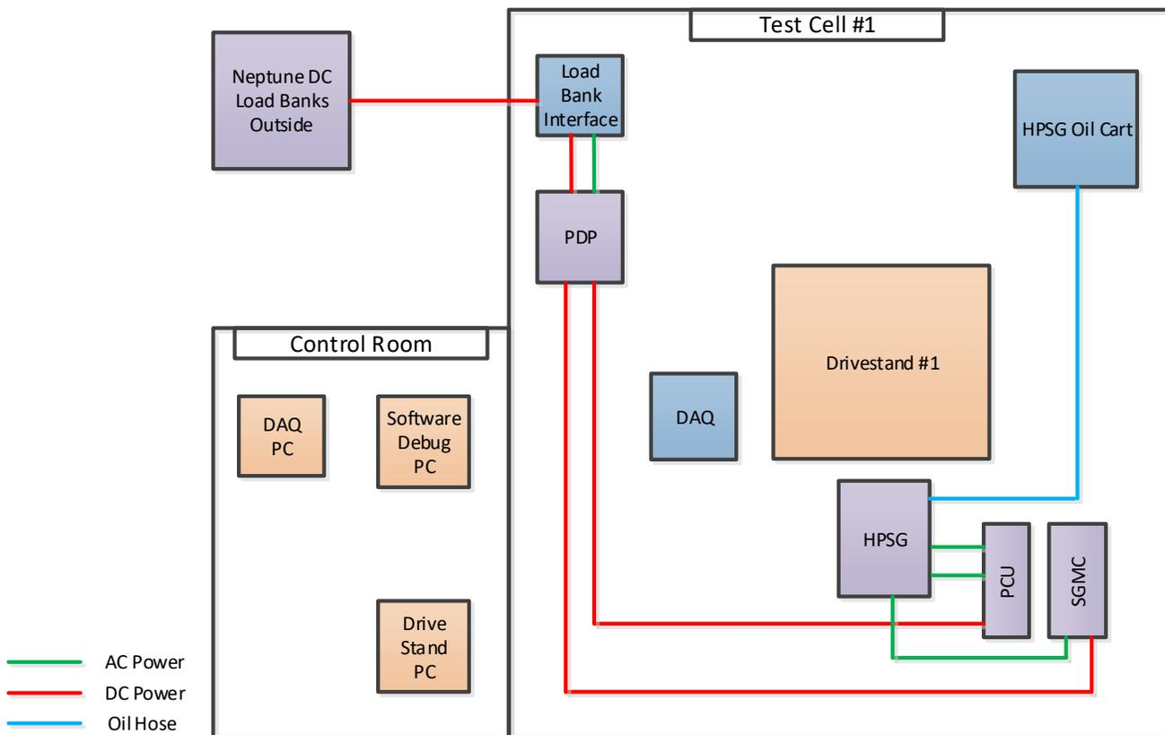
**Figure 7-1 - Test Cell Setup**
