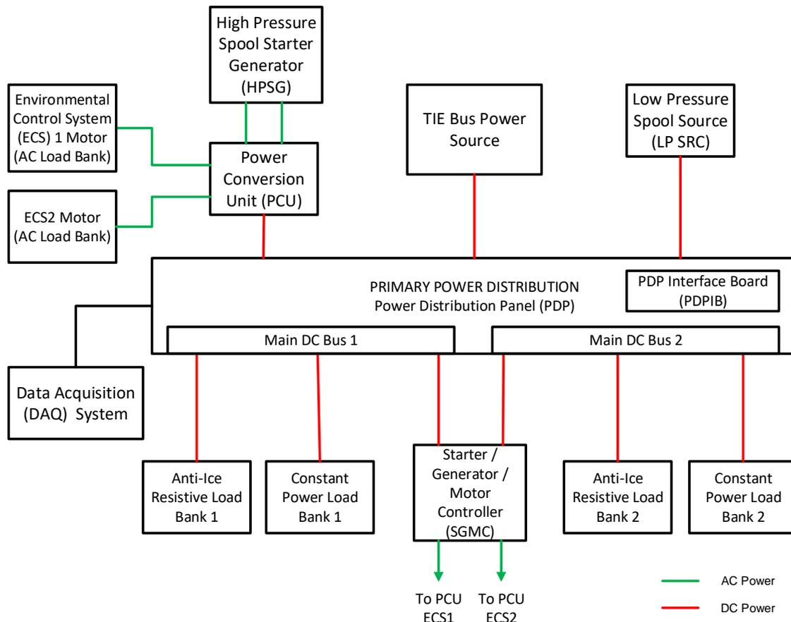
**Figure 3-1 – 300 kW Aircraft Architecture**
