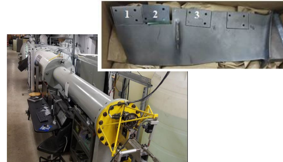
MDS Coating Fluid Erosion Test at Air Force Research Lab
