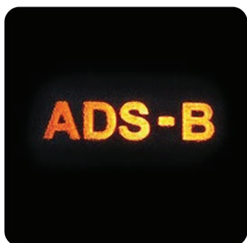
Figure 1 - Example of an ADS-B failure indication light.
