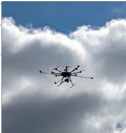
University of Kentucky's Octocopter drone research prototype in flight during the FOGMAP study. It carries pressure, temperature, humidity sensors, and four ultrasonic anemometers for wind and turbulence measurements.
