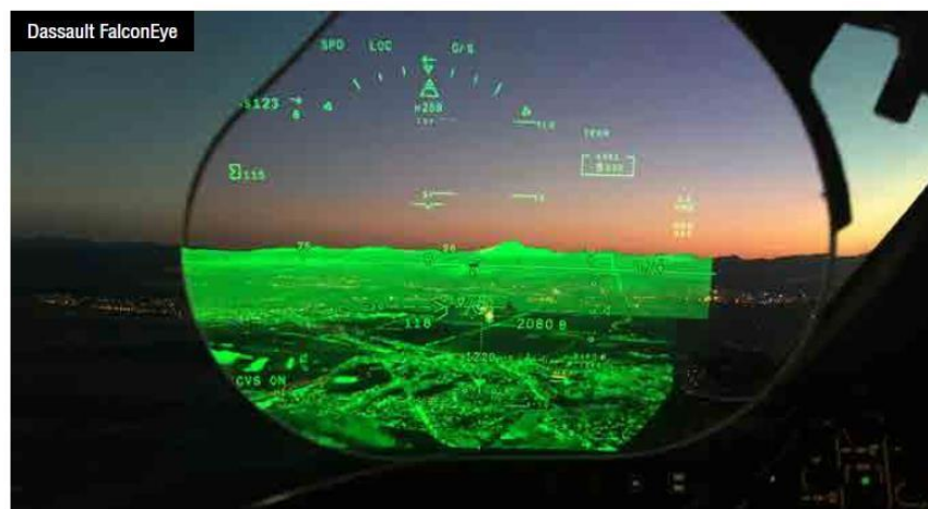
Figure 2-4. Example of CVS: Dassault FalconEye [20]
