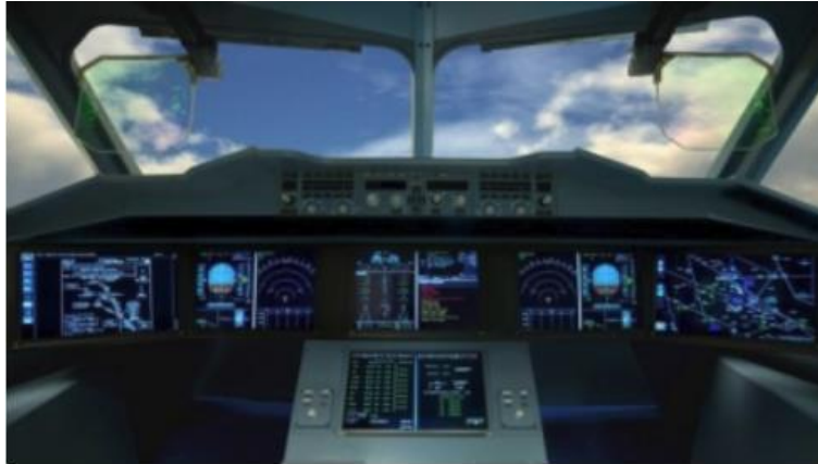
Figure 2-5. Example of a cockpit with a Thales Dual HUD installation [21]
