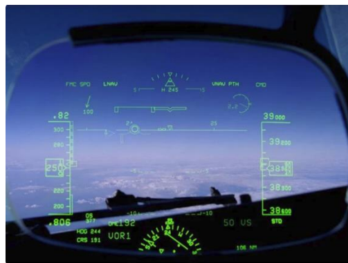
Figure 2-1. Example of information provided on a Collins Aerospace HUD [6]
