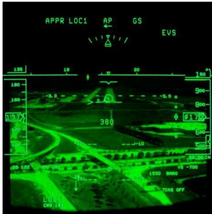
Figure 2-3. EFVS example from Collins Aerospace [15]
