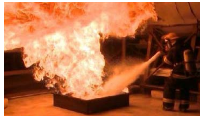
A 5 lb. CO2 fire extinguisher with Adiabatic expansion nozzle being tested against a 12 ½ sq/ft, Heptane fueled pan fire.
