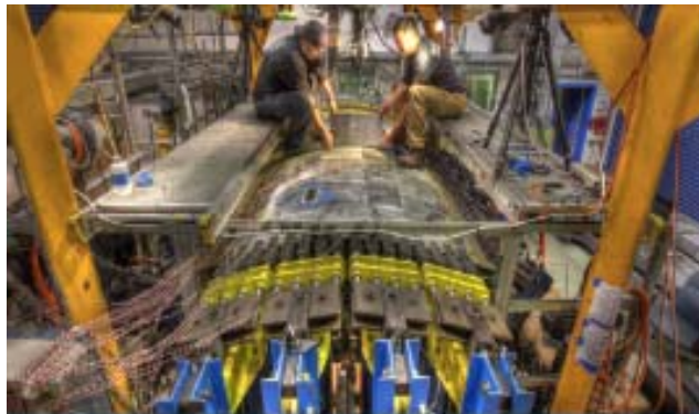
Installing of full-scale fuselage panel in the FASTER fixture – viewed from exterior surface
