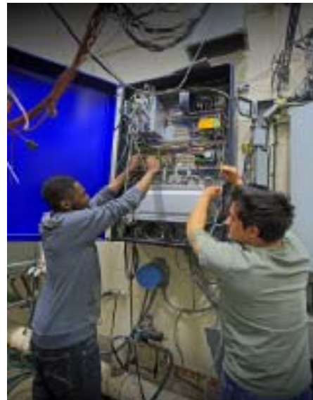
FAA licensed Airframe and Power Plant technicians connecting test cell sensor wiring and controls in preparation for testing
