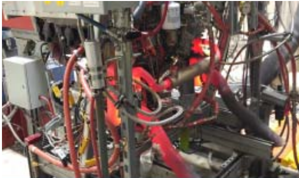
Engine showing glowing hot twin turbochargers during extreme testing of alternative fuels
