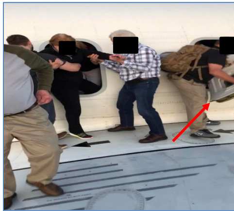
Figure 4 - Exit Door is Improperly Placed Outside, Creating Trip Hazard
