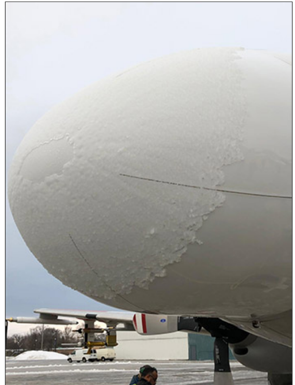
The ice-covered radome after a mission (Photo: FAA)
