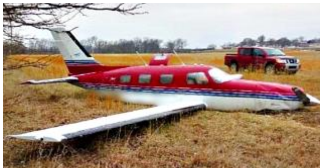
Aircraft after being unable to climb to 5,000 feet "We were starting to pick up moderate rime icing but the boots were still shedding the ice"
