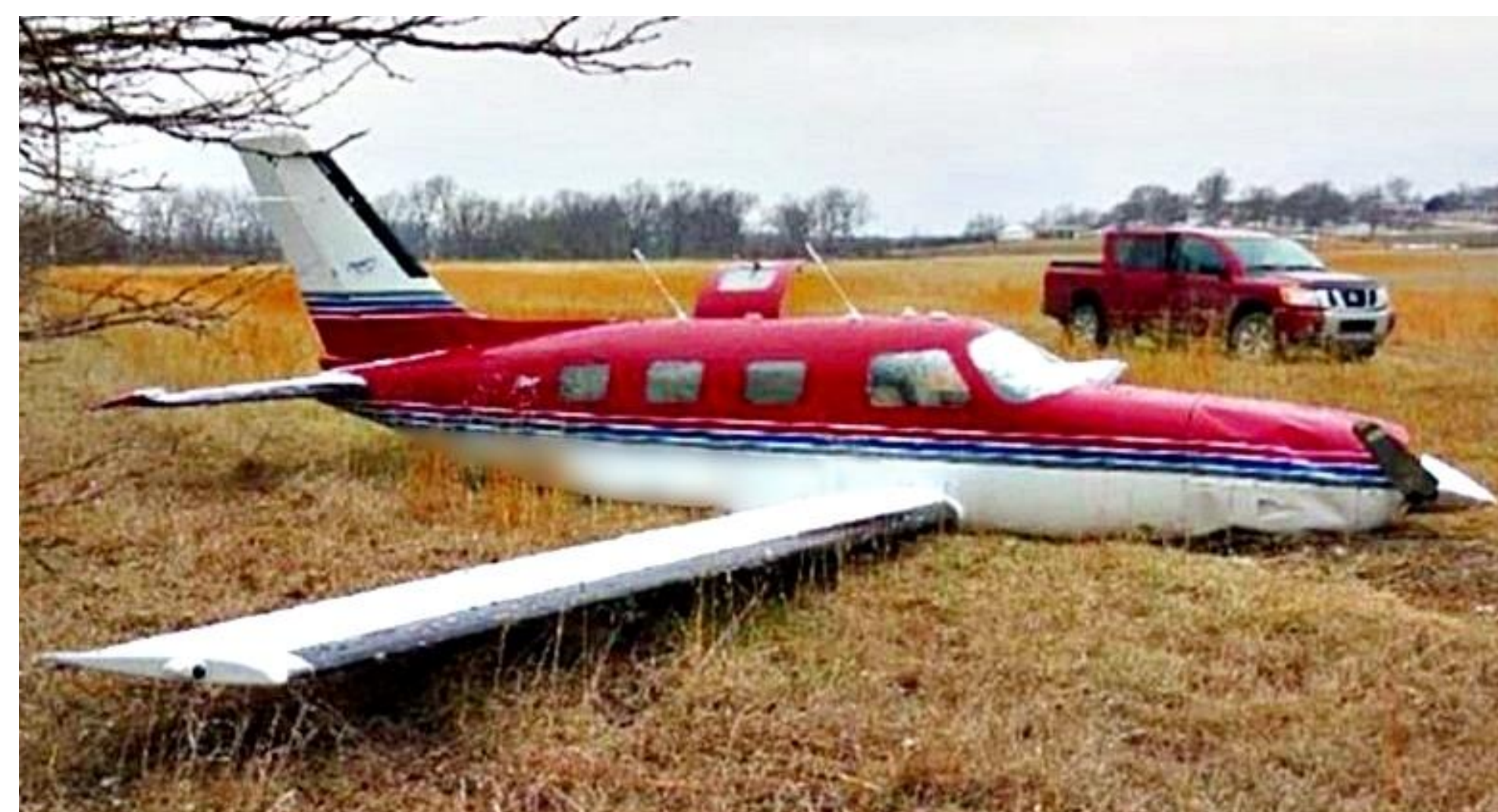
Aircraft after being unable to climb to 5,000 feet "We were starting to pick up moderate rime icing but the boots were still shedding the ice"
