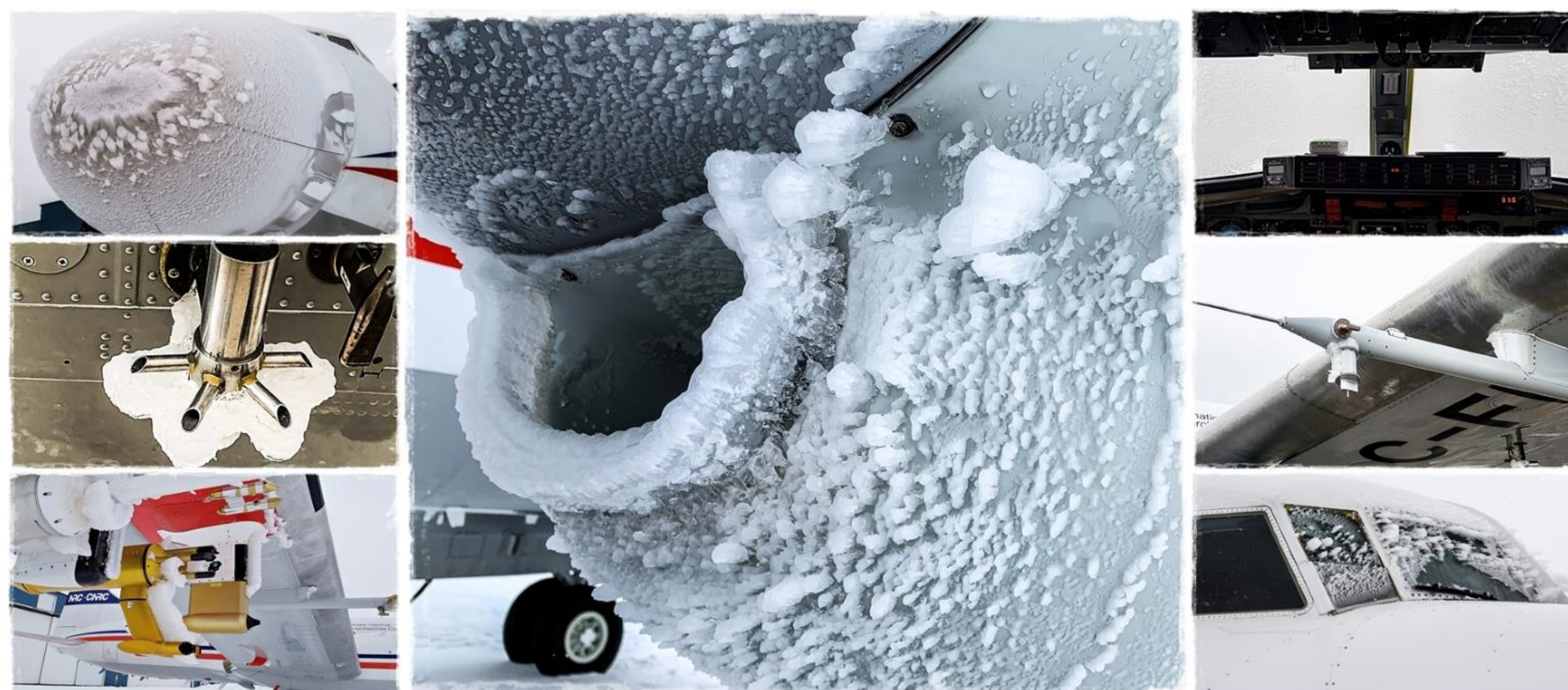
Ice accumulation on National Research Council of Canada (NRC) Convair-580 during In-Cloud Icing and Large-drop Experiment (ICICLE) Field Campaign
