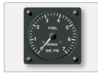
**Figure 14-84.** A differential fuel pressure gauge used on complex and high-performance reciprocating-engine aircraft compares the fuel inlet pressure to the air inlet pressure at the fuel metering device.
