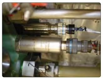
Figure 12-11. Temperature and quantity sensors.
