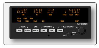
Figure 11-124. RNAV unit from a general aviation aircraft.
