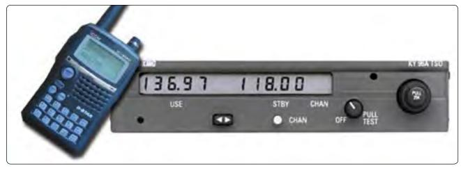
Figure 11-86. VHF aircraft communication transceivers.
