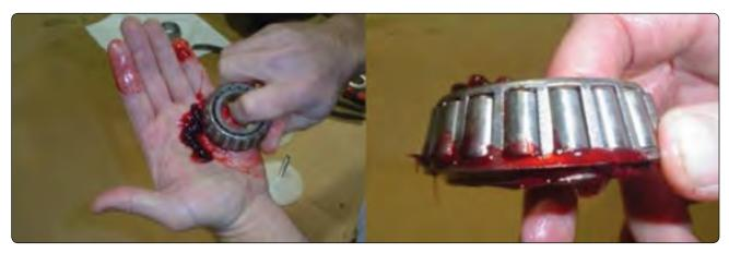
**Figure 13-45.** Packing grease into a clean, dry bearing can be done by hand in the absence of a bearing grease tool. Press the bearing into the grease on the palm of the hand until it passes completely through the gap between the rollers and the inner race all the way around the bearing.
