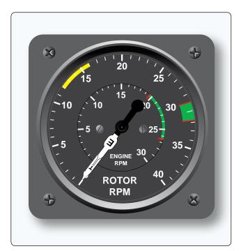
The tachometer probe's output signals need to be processed in a remotely located module. They must also be amplified to drive a servo motor type indicator in the cockpit. They may also be used as input for an automatic power control system or a flight data acquisition system. *[Figure 10-58]*
