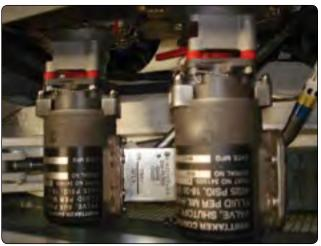
Figure 12-48. Shutoff valves.
