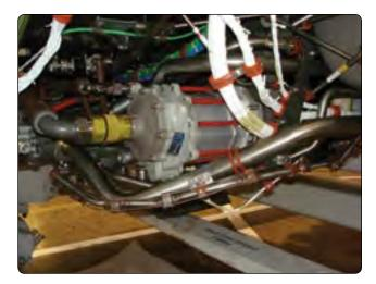
Figure 12-21. Engine-driven pump.
