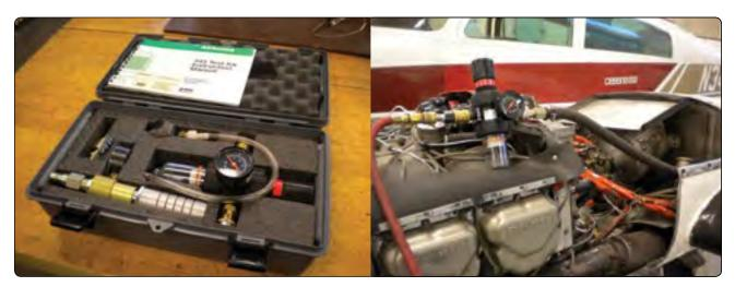
Figure 15-32. Test equipment used to test a wing deice system (left), and test equipment installed in the aircraft for testing (right).
