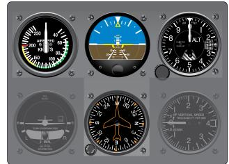
**Figure 10-4.** The basic T arrangement of analog flight instruments. At the bottom of the T is a heading indicator that functions as a compass but is driven by a gyroscope and not subject to the oscillations common to magnetic direction indicators.
