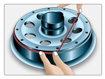
**Figure 13-153.** The wheel half O-ring for a tubeless tire wheel assembly must be in good condition and lubricated to seal for the entire life of the tire. The mating surfaces of the wheel halves must also be in good condition.
