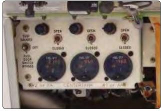
**Figure 14-106.** This panel at the pressure refueling station has valve position switches and quantity gauges to be used during refueling. Valve open position lights are adjacent to the switches for each tank.
