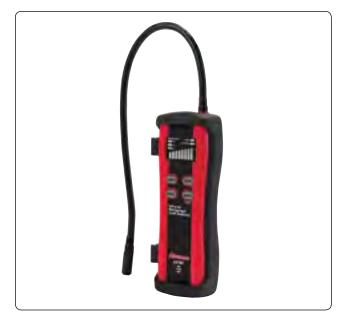
**Figure 16-92.** *This electronic infrared leak detector can detect leaks that would lose less than 1/4 ounce of refrigerant per year.*
