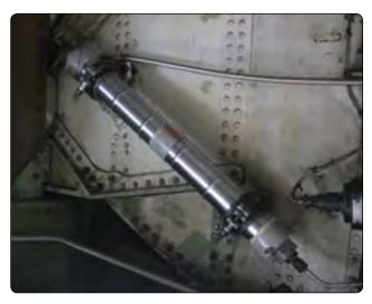
Figure 12-50. Cylindrical accumulator.
