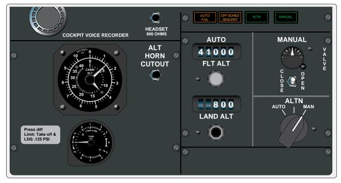
Figure 16-53. This pressurization panel from an 800 series Boeing 737 has input selections of flight altitude and landing altitude.
