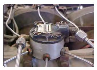
Figure 14-15. A fuel distribution manifold for a fuel-injected engine.
