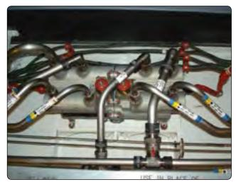
Figure 12-35. Four-way servo control valve.
