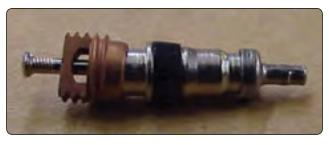
**Figure 13-148.** The tire valve core should be removed after the tire is completely deflated and before the tire and wheel assembly is removed from the aircraft.
