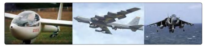
**Figure 13-5.** Tandem landing gear along the longitudinal axis of the aircraft permits the use of flexible wings on sailplanes (left) and select military aircraft like the B-52 (center). The VTOL Harrier (right) has tandem gear with outrigger-type gear.
