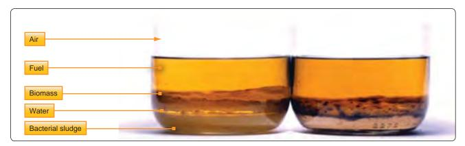
Figure 14-96. This fuel-water sample has microbial growth at the interface of the two liquids.
