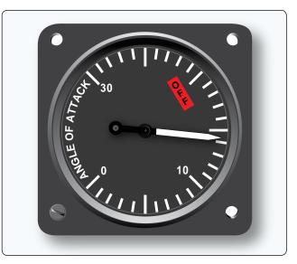
Figure 10-63. Angle of attack indicator.
