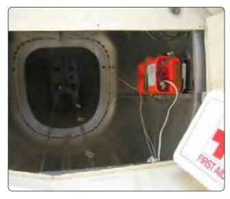
**Figure 11-149.** An emergency locator transmitter (*ELT*) mounting location is generally far aft in a fixed-wing aircraft fuselage in line with the longitudinal axis. Helicopter mounting location and orientation varies.
