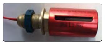
**Figure 14-103.** A float switch installed in a fuel tank can close the refueling valve when the tanks are full during pressure fueling of an aircraft. Other more sophisticated automatic shutoff systems exist.
