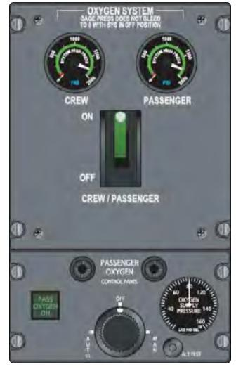
**Figure 16-16.** *The crew can deploy passenger emergency continuousflow oxygen masks and supply with a switch in the cockpit.*
