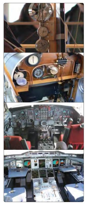
**Figure 10-1.** From top to bottom: instruments of the Wright Flyer, instruments on a World War I era aircraft, a late 1950s/early 1960s Boeing 707 airliner cockpit, and an Airbus A380 glass cockpit.
