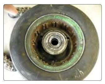
**Figure 13-60.** *Keys on the inner wheel half of an aircraft wheel used to engage and rotate the rotors of a disc brake.*
