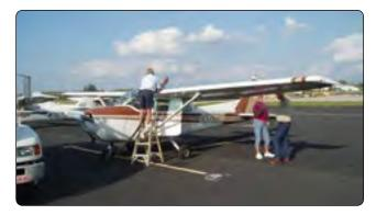
Figure 14-105. Over-the-wing refueling a Cessna.
