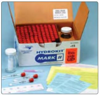
Figure 14-98. This kit allows periodic testing for water in fuel.
