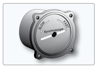
**Figure 10-59.** *This synchroscope indicates the relative speed of the slave engine to the master.*
