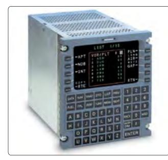
Figure 10-127. The control display unit (CDU) of an FMS.
