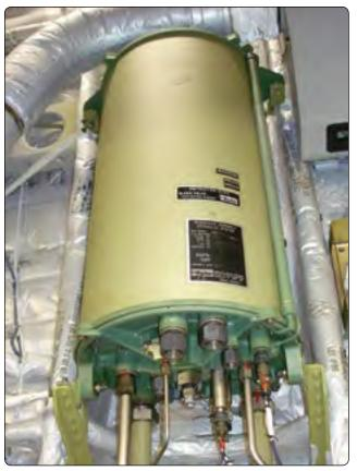
Figure 12-9. Air-pressurized reservoir.
