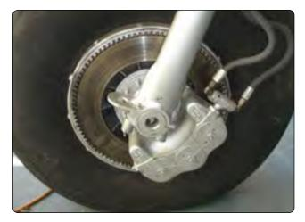
**Figure 13-78.** A single disc brake is a floating-disc, fixed caliper brake.
