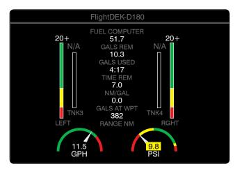
**Figure 14-85.** An electronic display of fuel parameters, including fuel pressure.
