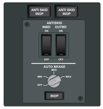
Figure 13-105. Antiskid switches in the cockpit.
