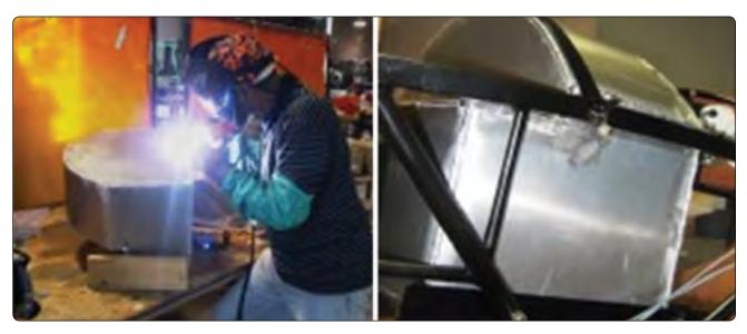
Figure 14-90. A rigid removable fuel tank with welded seams is repaired by welding.
