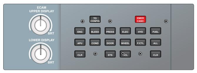
Figure 10-121. An ECAM display control panel.
