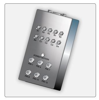
Figure 11-129. A handheld transponder test unit.
