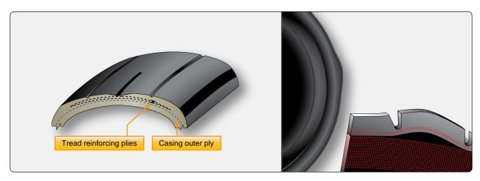
Figure 13-141. Bulges and tread separation are cause for removal of a tire from service.
