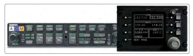
**Figure 11-73.** An audio panel in a general aviation aircraft integrates the selection of several radio-based communication and navigational aids into a single control panel (left). A digital tuner (right) does the same on a business class aircraft and allows the frequency of each device to be tuned from the same panel as well.
