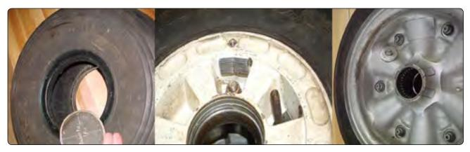
**Figure 13-159.** A tire balancing patch (left), adhesive wheel weights (center), and a bolted wheel weight (right) are all used to balance aircraft tire and wheel assemblies per the manufacturer's instructions.
