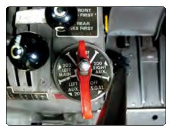
**Figure 14-38.** *Detents for each position, an indicating handle, and labeling aid the pilot in knowing the position of the fuel valve.*
