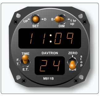
Figure 10-132. A typical aircraft electronic clock.
