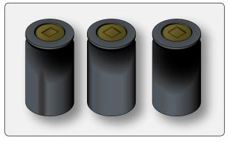
**Figure 13-66.** Overheating caused by lack of sufficient lubrication results in a bluish tint to the metal surface. The ends of the rollers shown were overheated causing the metal to flow and deform, as well as discolor. The bearing cup raceway is usually discolored as well.
