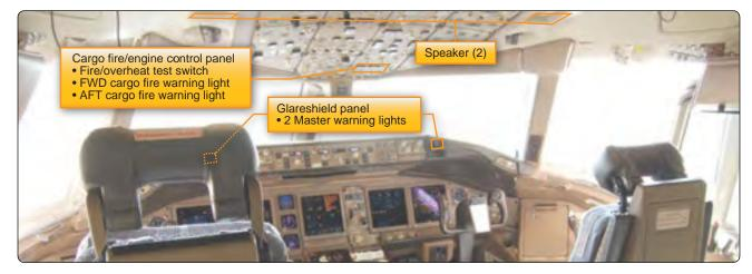
Figure 17-18. Cargo fire detection warning.
