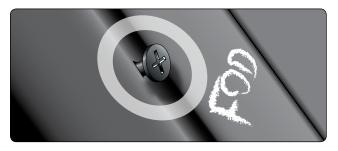
**Figure 13-137.** *Marking of damaged area to enable closer inspection.*
