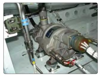
Figure 12-22. Electrically-driven pump.
