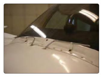
Figure 15-46. Chemical deicing spray tubes.
