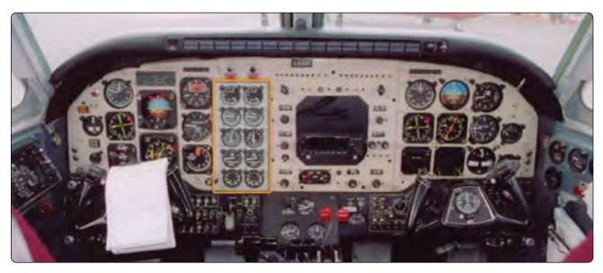
Figure 10-7. An engine instrumentation located in the middle of the instrument panel is shared by the pilot and co-pilot.
