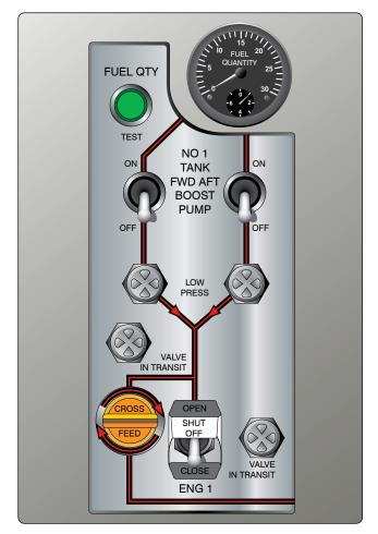
**Figure 14-88.** Valve-in-transit lights are used on this section of a transport category aircraft fuel panel. Low boost pump pressure lights that look the same are also on the panel.
