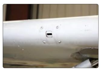
**Figure 10-61.** A reed-type stall warning device is located behind this opening in the leading edge of the wing. When the angle of attack increases to near the point of a stall, low-pressure air flowing over the opening causes a suction, which audibly vibrates the reed.
