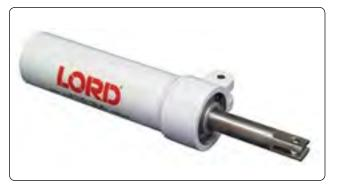
**Figure 13-56.** A non-hydraulic shimmy damper uses a rubber piston with lubricant that dampens via motion against the inner diameter of the unit housing.
