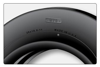
**Figure 13-132.** A sidewall vent marked by a colored dot must be kept free from obstruction to allow trapped air or nitrogen to escape from the carcass plies of the tire.
