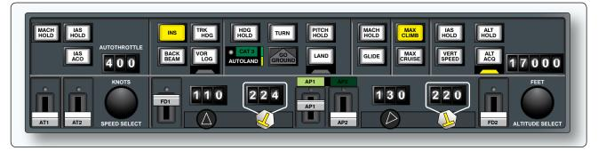
**Figure 10-112.** The AFCS control panel commands several integrated systems from a single panel including: flight directors, autopilots, autothrottles, autoland, and navigational aids. Mode selections for many features are made from this single interface.
