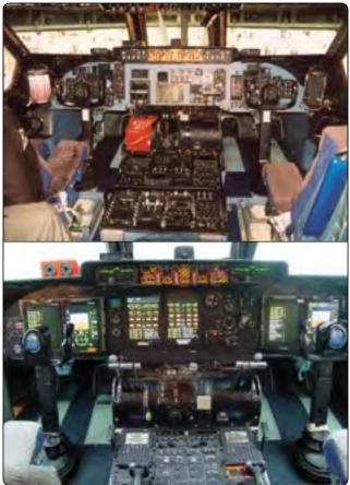
**Figure 10-2.** *A conventional instrument panel of the* C-5*A Galaxy (top) and the glass cockpit of the* C-5*B Galaxy (bottom).*
