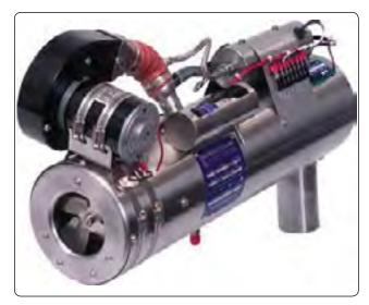
Figure 16-99. A modern combustion heater.
