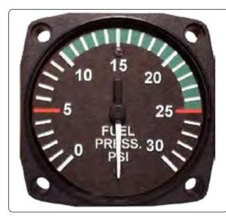
Figure 10-17. A typical analog fuel pressure gauge.
