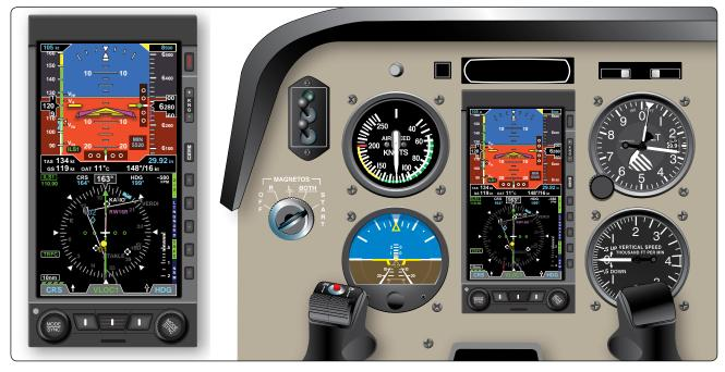
Figure 11-71. A retrofit digital data display.
