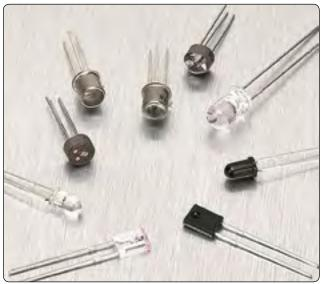
Figure 11-40. Phototransistors.
