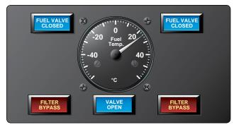
**Figure 14-64.** *A Boeing 737 cockpit fuel panel showing illuminated valve position indicators and fuel filter bypass lights. The fuel temperature in tank No.1 is also indicated.*
