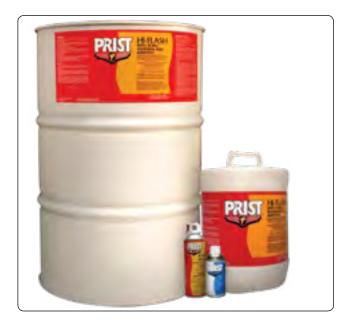
**Figure 14-9.** Fuel anti-icing products, such as Prist<sup>®</sup>, act as antifreeze for any free water in aircraft fuel. They dissolve in the water and lower its freezing point to prevent ice crystals from disrupting fuel flow.
