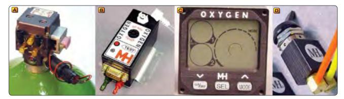
**Figure 16-25.** The key components of a built-in electronic pulse demand oxygen metering system: (A) electronic regulator, (B) oxygen station distributer unit, (C) command/display unit, (D) emergency bypass switch.
