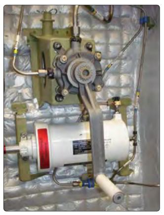
Figure 12-20. Rotary hand pump.
