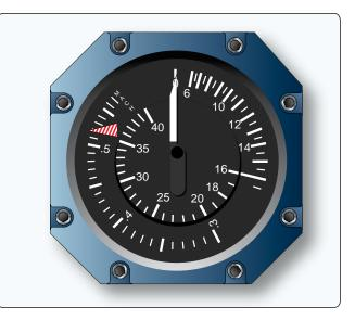
**Figure 10-46.** A combination Mach/airspeed indicator shows airspeed with a white pointer and Mach number with a red and white striped pointer. Each pointer is driven by separate internal mechanisms.
