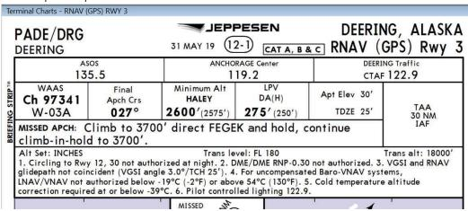
When both temperature limits appear on the same chart and they are different, it has led to pilot confusion in terms of applying temperature compensation. The reason for differences is because of the differing purpose for each limit, as follows:
