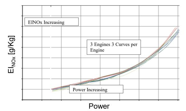
$\mathsf{EI}_{\mathsf{NOx}}$  vs. Thrust for a Modern Rich Burn Combustor Led to the development of Lean Burn Combustor
