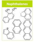
Jet fuel is composed of up to ~ 2% naphthalene, but **fuels absent naphthalene have** ~ **15 – 40% lower nvPM emissions**, i.e., napthalenes have a disproportionate contribution to nvPM emissions
