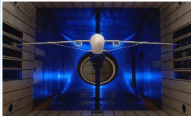
Transonic Truss-Braced Wing 5-10% fuel burn benefit
