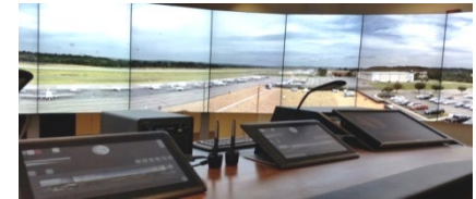
Remote Tower Displays of Airfield w/ Controller positions
