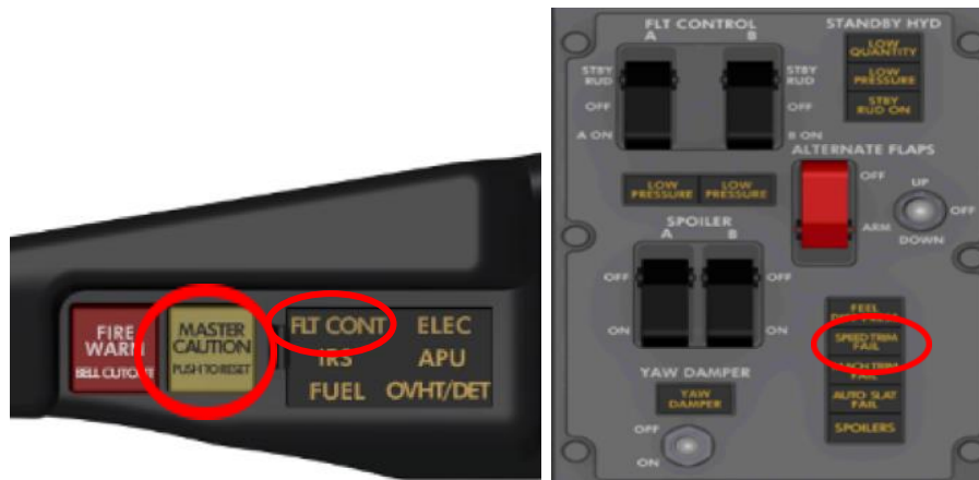
FIGURE 2 SPEED TRIM FAIL ANNUNCIATION
