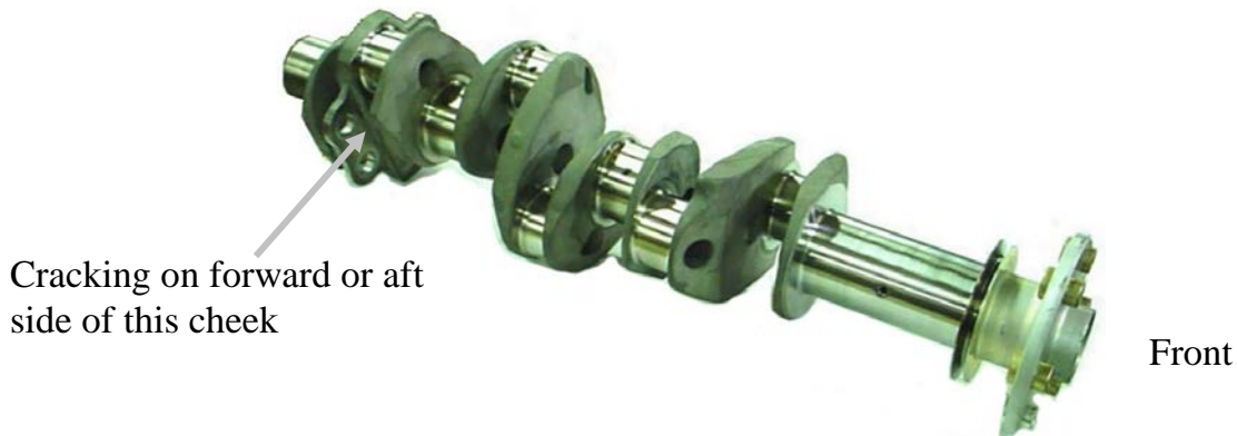
Location of Crankshaft Cracking (3-D View of Complete Crankshaft) Figure 3-1
