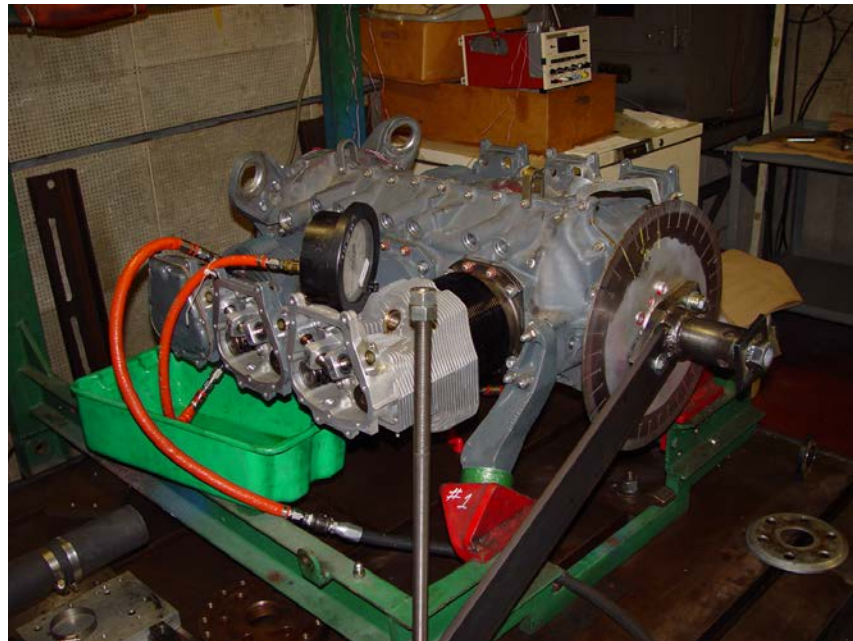
Crankshaft Static Stress Test Rig Figure 6-3
