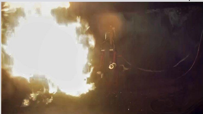
Researchers test an aerosol can simulator explosion in a DC-10 cargo compartment.
