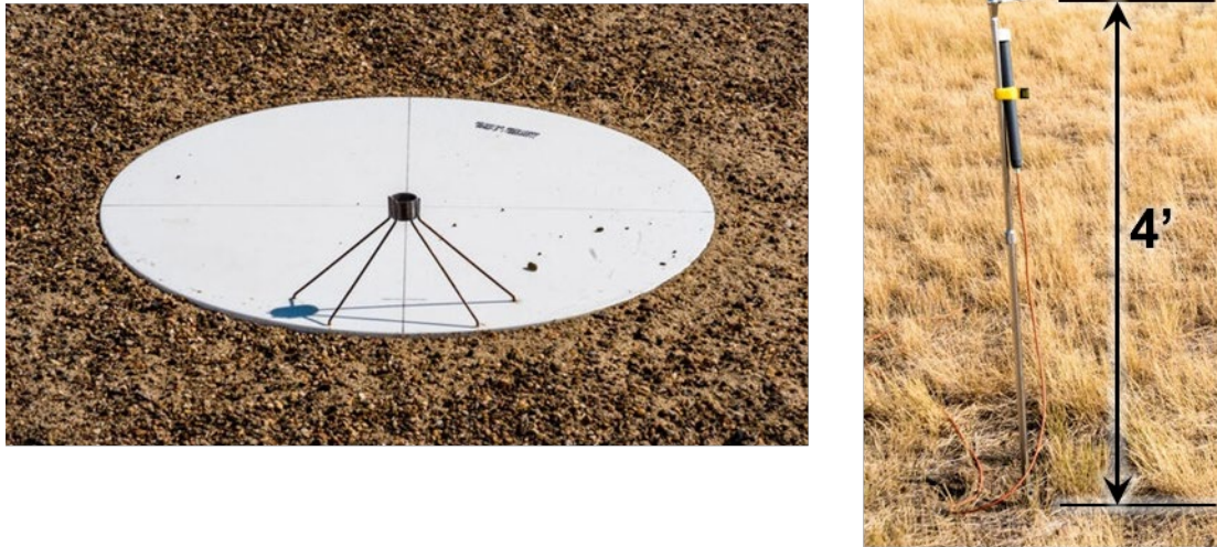
Figure 5-7 - SAE Ground Plane Microphone Base and Pole Microphone
