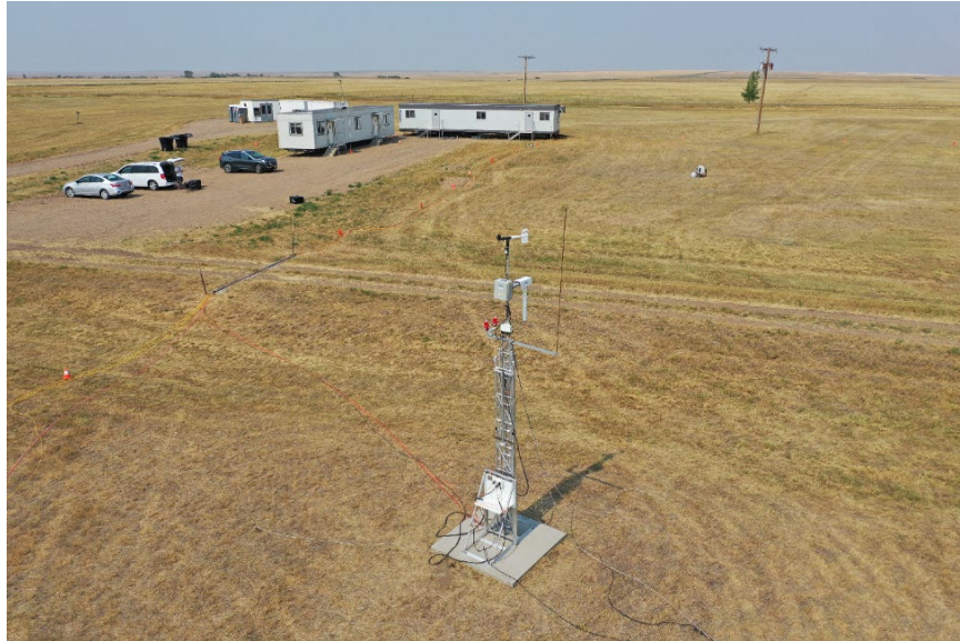
Figure 5-4 - 10m Surface Weather Station, SWX, with the data acquisition and analysis trailers in the background
