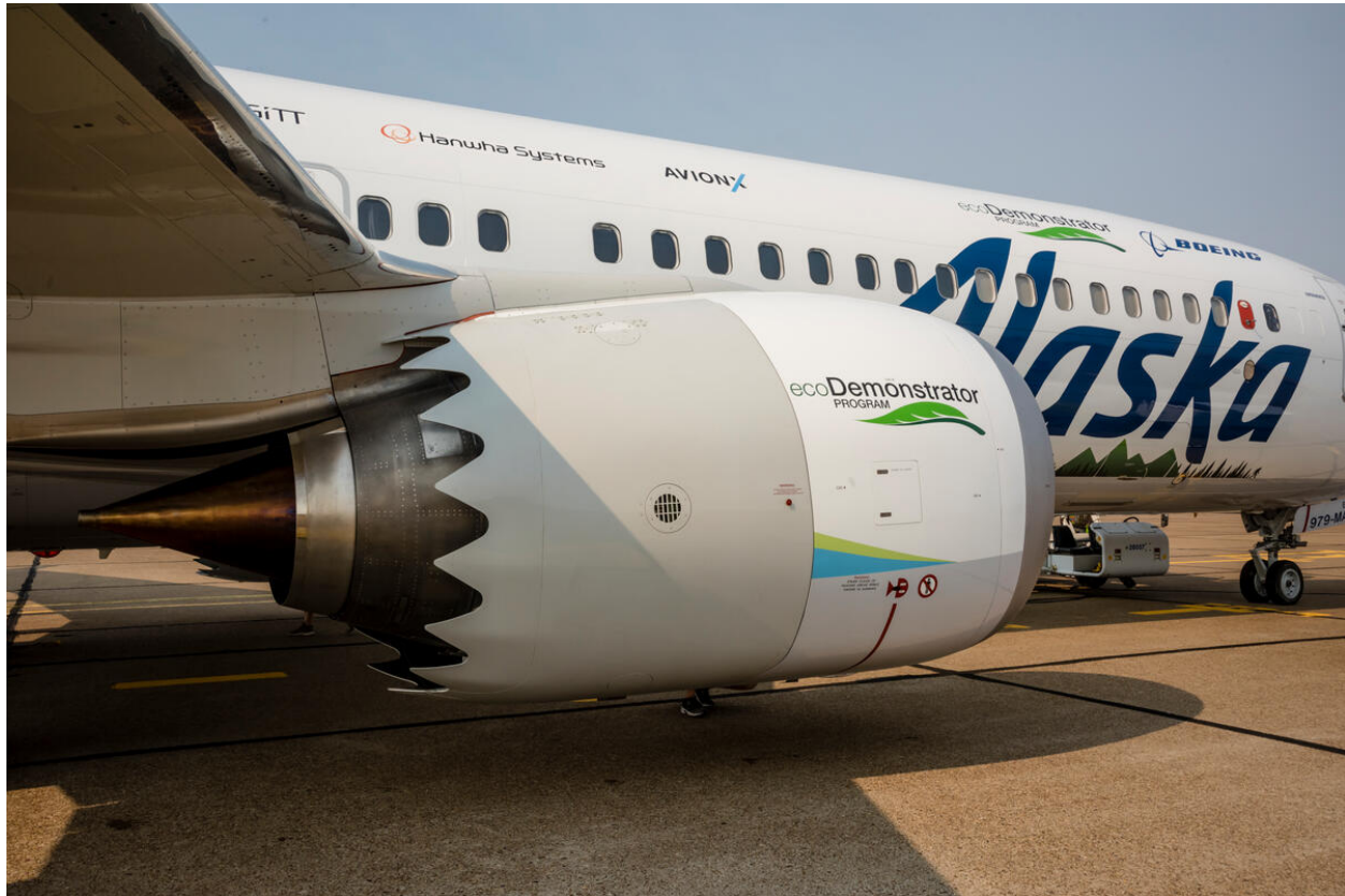
Figure 6-2 - Right Engine outfitted with test hardware
