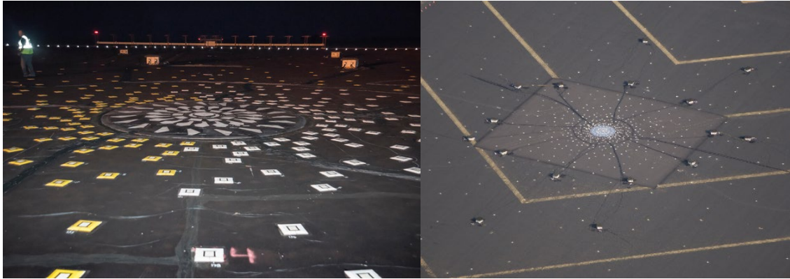
Figure 5-9 - Phased Array Microphones, power supplies, and locators
