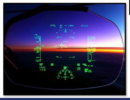
An EFVS includes the display element, sensors, computers, power supplies, indications, and controls.
