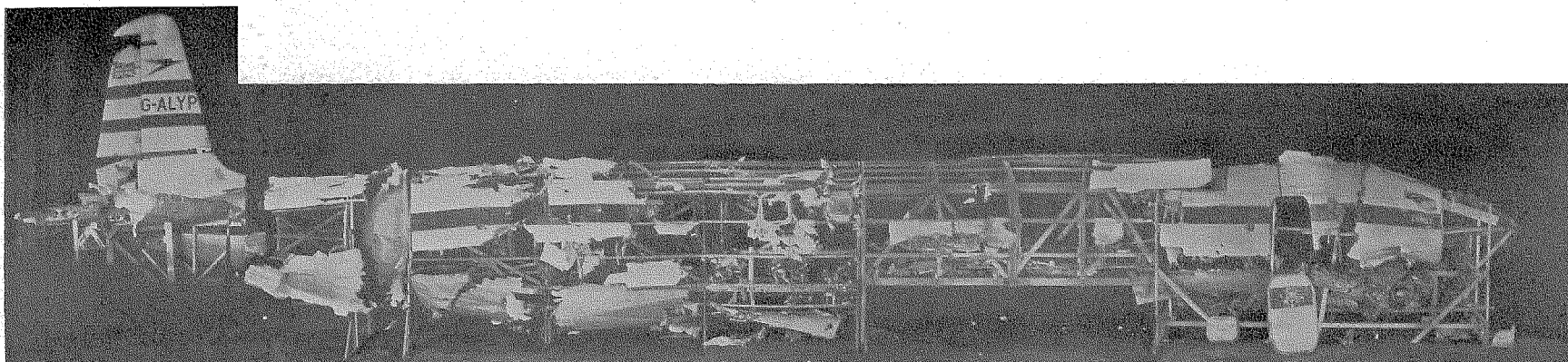
FIG. 4. RECONSTRUCTION OF FUSELAGE AND TAIL UNIT WRECKAGE—G-ALYP.
