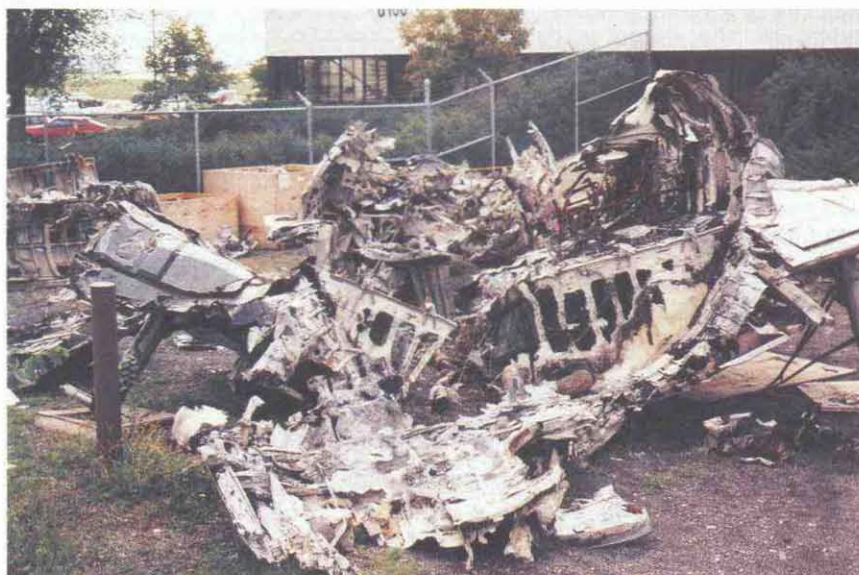
Fuselage view from rear showing burnt out cabin area.
