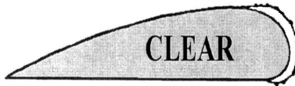
FIGURE 5. CLEAR ICE BUILDUP WITH HORNS
