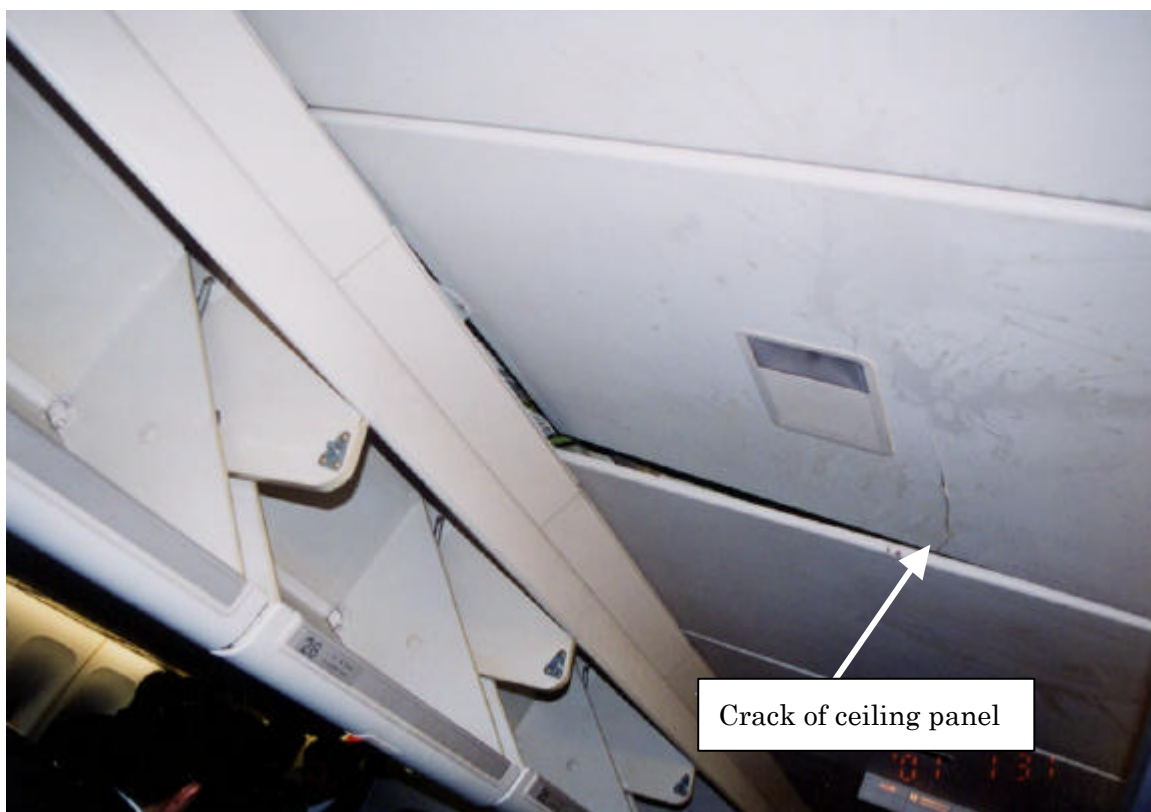
The damage of ceiling panel over right side pass way seat No. 26(view from backward)
