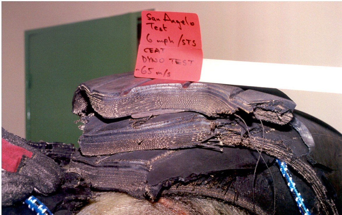
Figure 50: Cuts in various Concorde tyres
